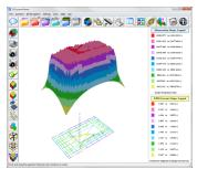
packages. Furthermore, all computation results pertaining to the system configuration can be displayed right on the system component itself in vivid spot colors that reflect the intensity of the displayed quantity (such as leakage and longitudinal currents, ground potential rises (GPR), etc.).
